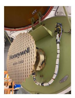
Radar image of mounted RDR-7000 in place of former radar system
